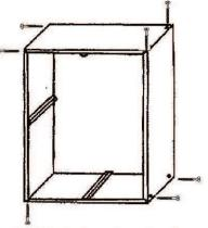
Attach the four pieces together with eight 2" screws. Do not tighten them all the way until diamond is fully assembled.
