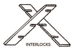
3. Assemble two long interlocks and place into constructed box.
