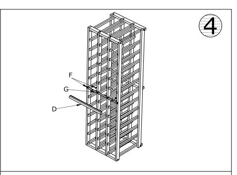
4. After all set stand this part then install metal Front Support(G) with screw (F) then install Center front Trim (D) with screw (F) from inside the rack, see picture (4).
