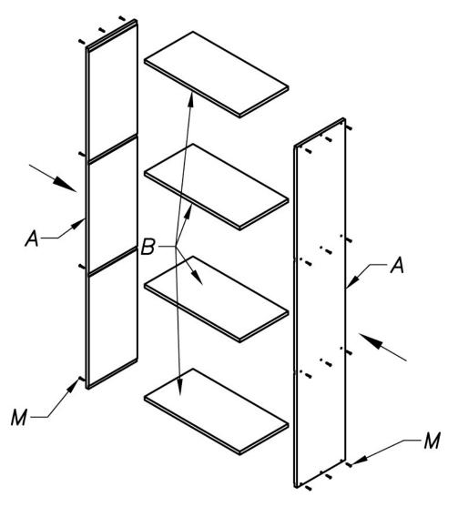
1. Attach the right and left boards (A) to the center boards (B) using screws (L). Do not tighten screws completely. This will allow easier installation of cross boards.
