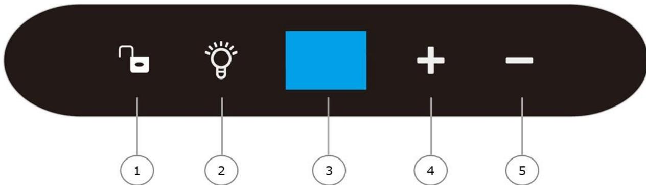
1. LOCK: Press and hold for 2 seconds to Lock or Unlock the control panel.
