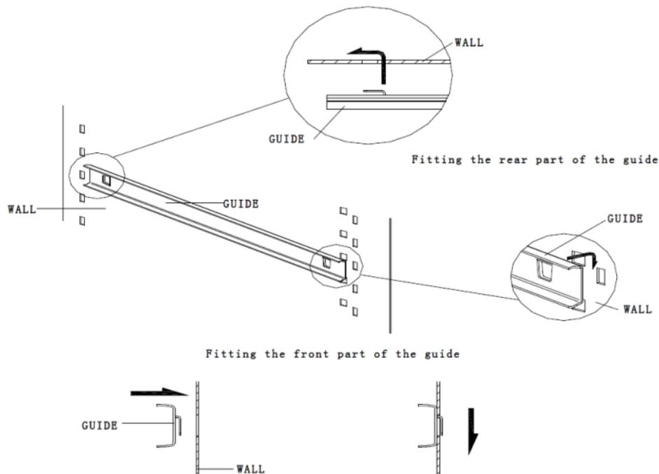
Reposition guide rail to the new location and reinstall in reverse order.
